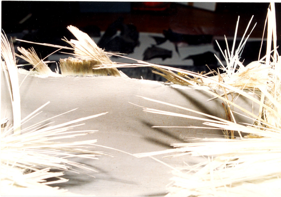
40. Close-up view of the failed tank edge looking at the right side of the tank with the forward end toward the right side of the photograph
